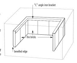
Now place one extra whole and one half firebrick on either side of the firebox to complete the installation of the firebricks. (i.e. two and a half each side and remainder on the back wall.)
