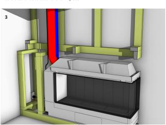
Install electrical, network connections, and gas supply.
