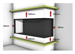
Ensure all clearances are met to any combustible or heat sensitive materials in front, above, to the side, or below the fireplace viewing area. Following these clearances, will allow the use of standard building materials, whether combustible or non-combustible. It is recommended to keep furnishings at least **1m** from the front of the fireplace
