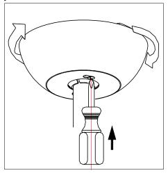
Carefully put the screw cap on using the piece of magnetic supplied.
