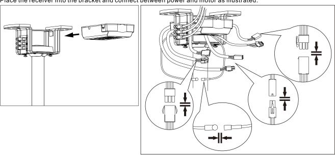
Wire up the receiver with quick connectors and insert into the mounting bracket. Please make sure the antenna wire has been safely folded inside the canopy cover before final assembly (DO NOT cut the antenna wire)
